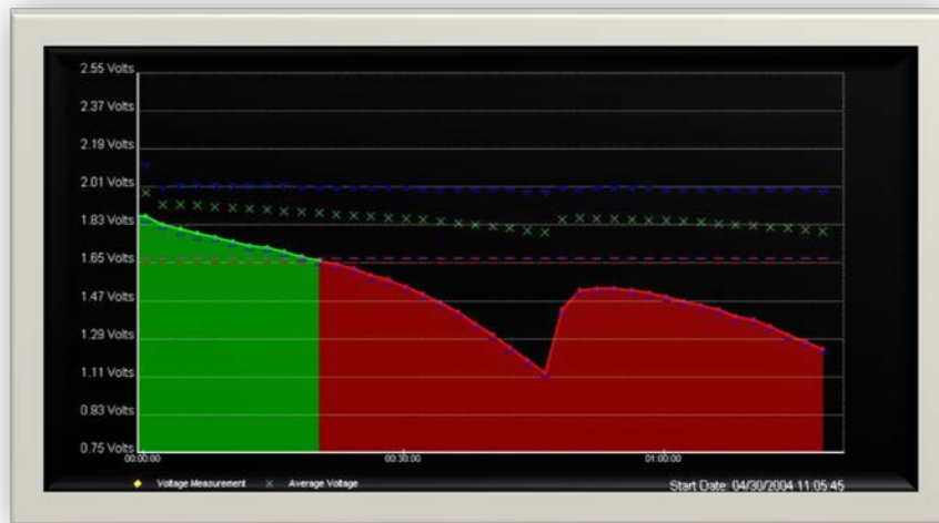
Snap shot of unit voltages at Low Voltage Cut off
